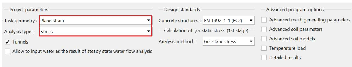
The screenshot shows the 'Settings' card in the GEO5 software interface. It is divided into three main sections: Project parameters, Design standards, and Advanced program options.
